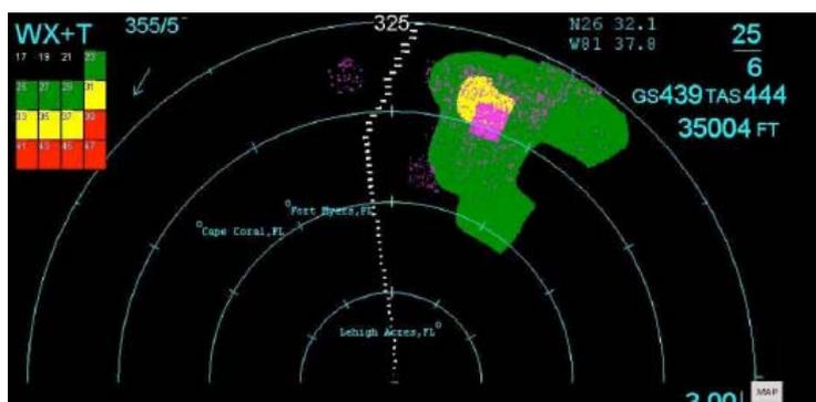
Figure 6: Example of E-Turb Radar Scan
